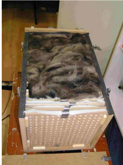
Figure 18: Damping by flow-resistor covered with fiber-cloth and the remainder of the pipe filled with long-fiber sheep-wool.
