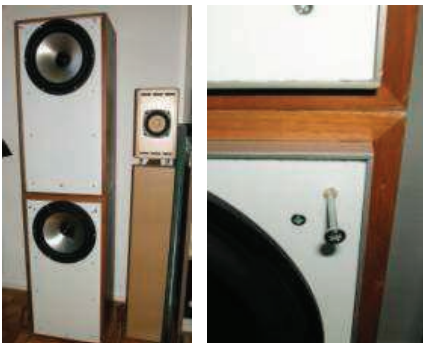
The two sub's next to the Solo-103. Note the height adjustable "spike".
