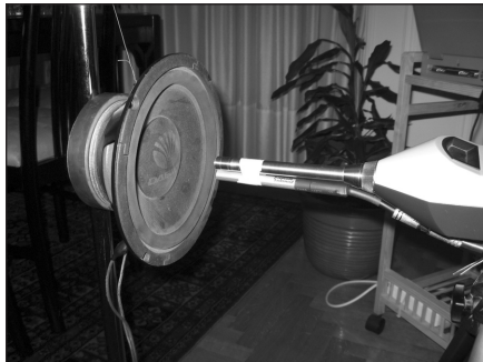
PHOTO 2: The test setup for the measurement of the low-frequency response using an 8" driver.
