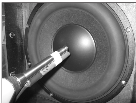
PHOTO 3: The test setup for the measurement of the low-frequency response and the distortion using a 10" driver.
