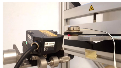
Fig. 10: Measurement of the side VCF displacement.
