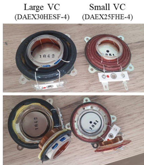
Fig. 2: Examples of the chosen exciters with large voice coil and with small voice coil.
