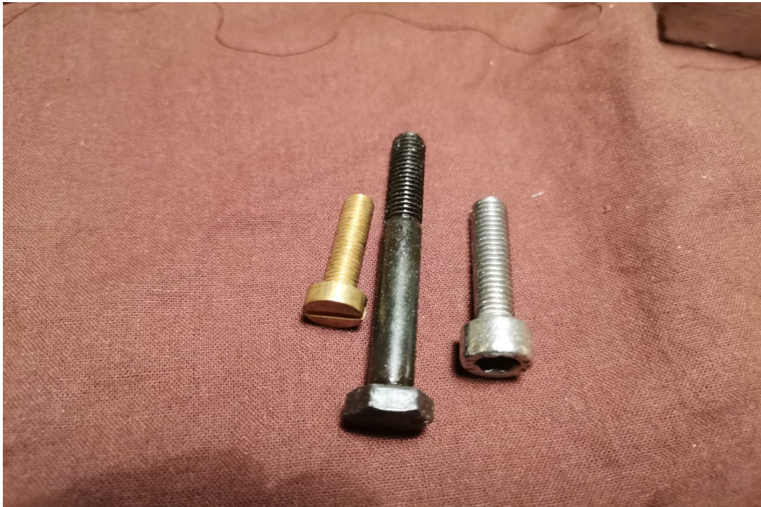
Figura 4: The three screws used for test, M6 size, brass, normal steel and stainless.
