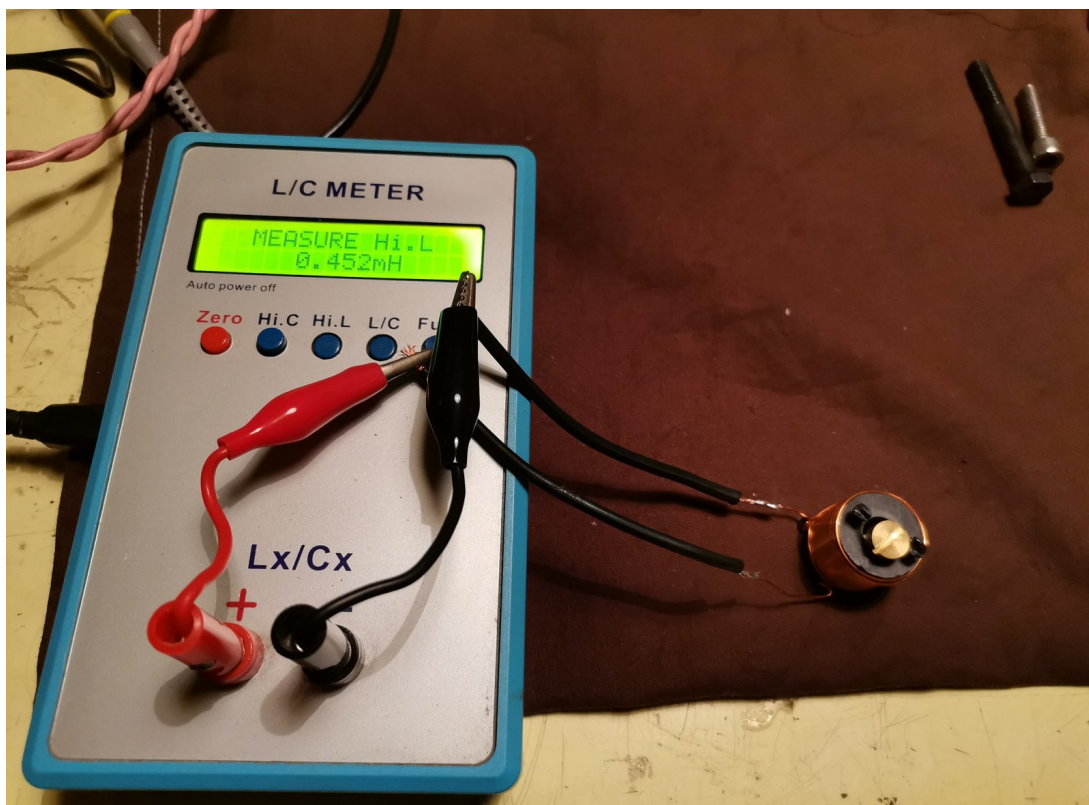
Figura 5: Brass core inserted, the inductance value is 0,452mH
