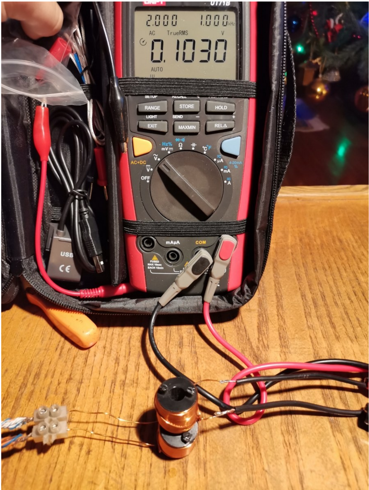
Figura 24: True-rms multimeter shows 0,103v rms at 1khz.
