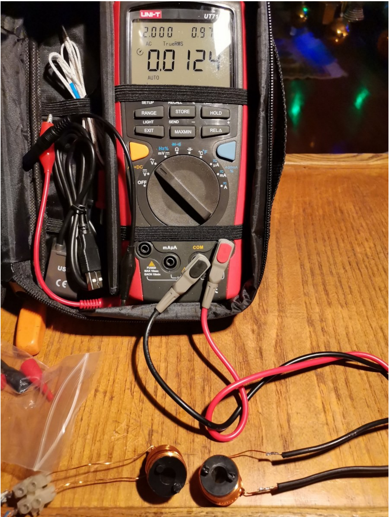
Figura 27: Coils close together placed with different position, the cross-talk is limited.
