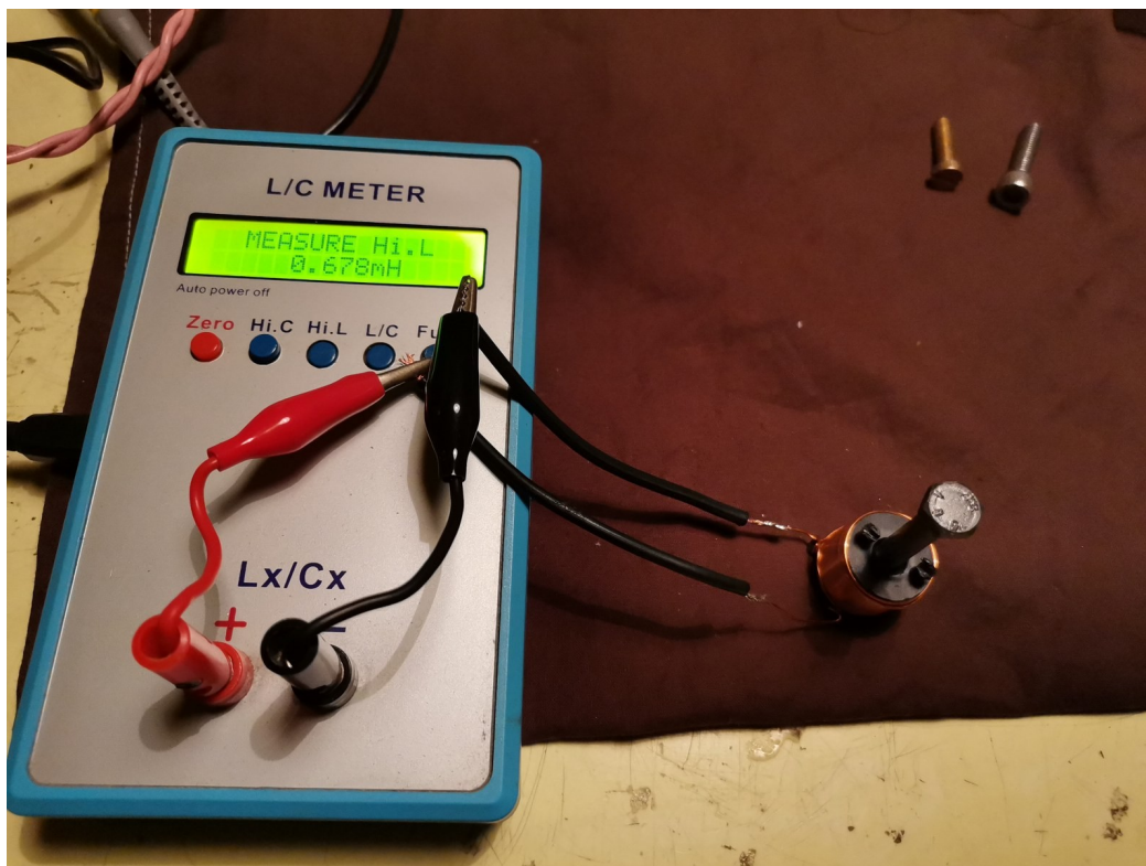
Figura 7: Steel inserted, the inductance value is 0,678mH
