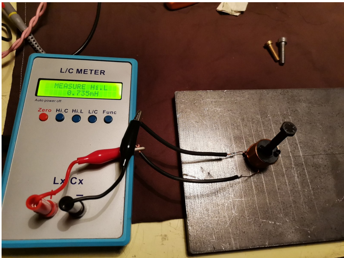
Figura 13: Steel core on steel plate, value 0,735mH.
