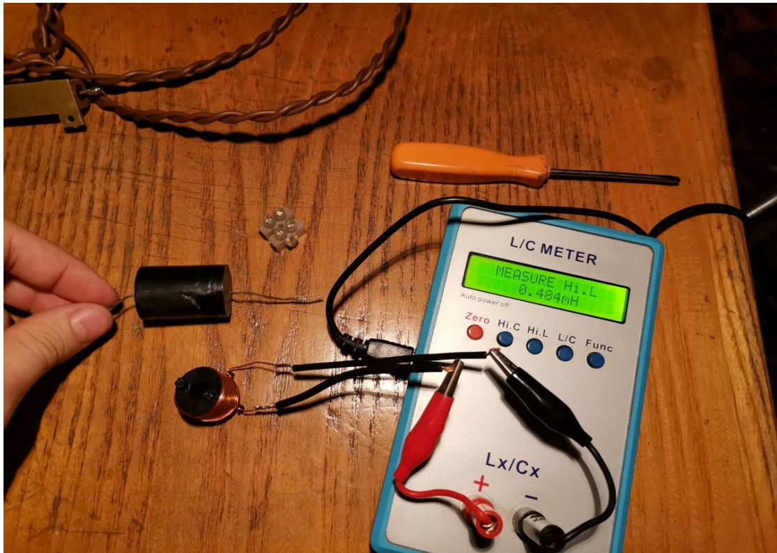
Figura 29: MKP cap, 8,2uF, non metallic shell has no influence on the inductance.
