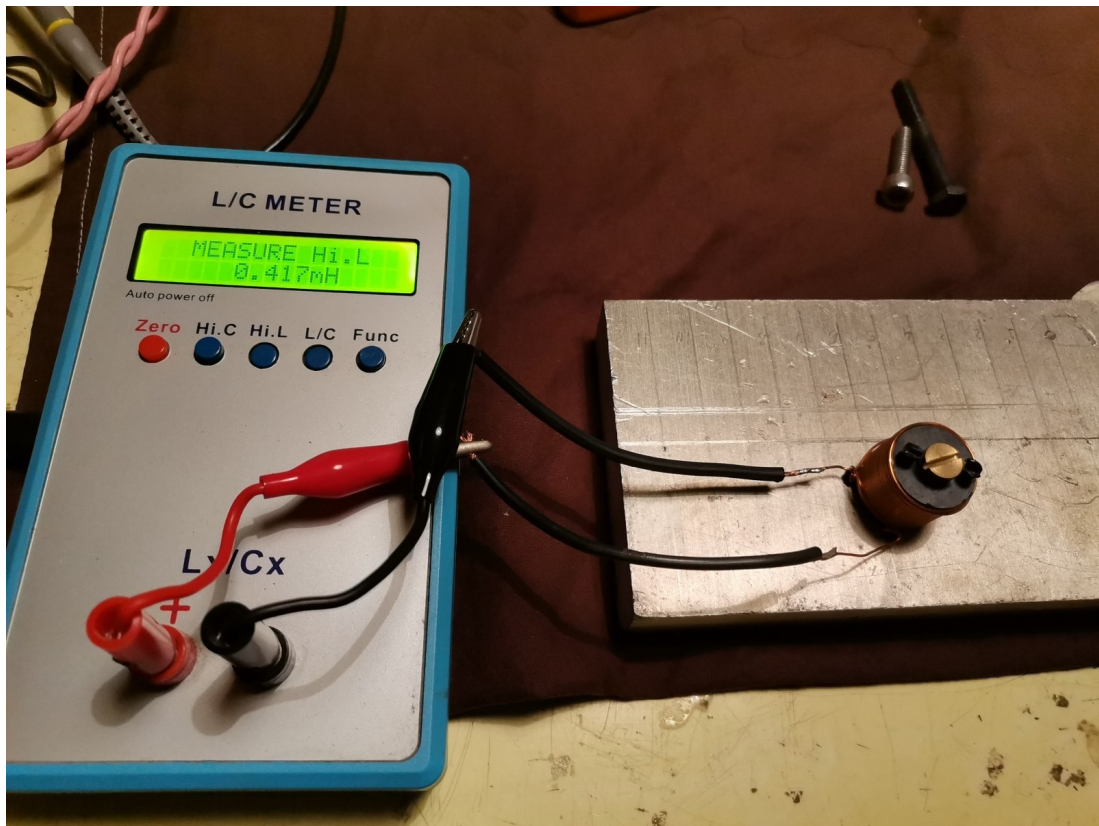
Figura 8: Brass core on aluminum plate, value 0,417mH
