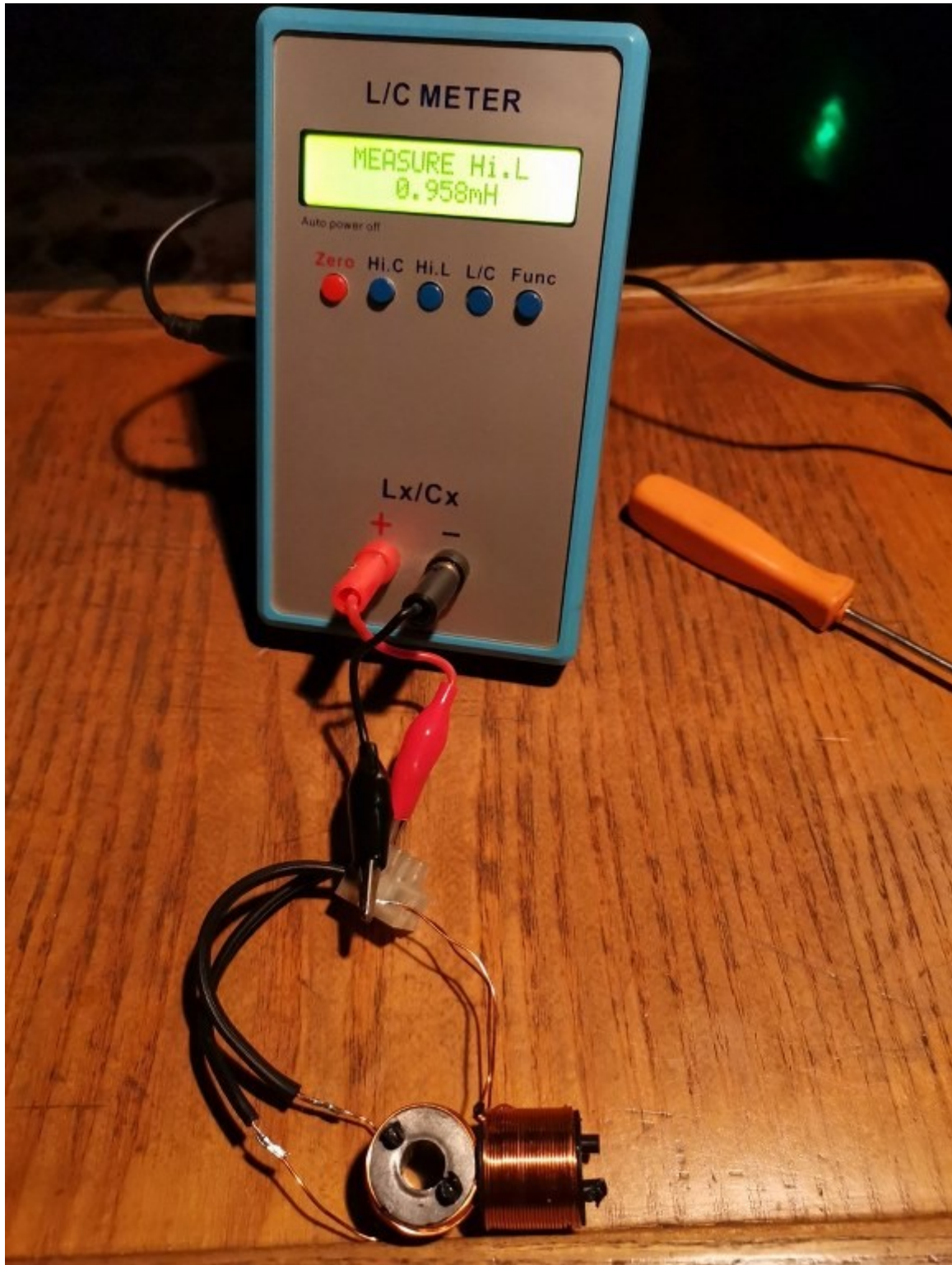
Figura 20: Coils closed together, perpendicular axis, 0,950mH.
