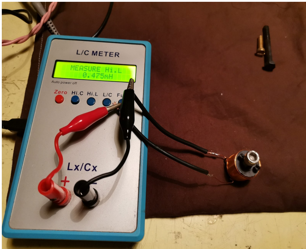
Figura 6: Stainless steel inserted, the inductance value is 0,475mH.
