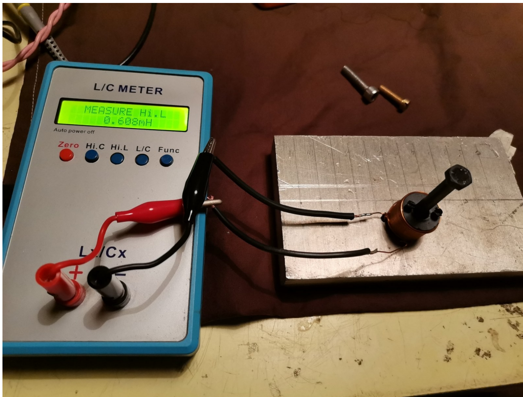
Figura 10: Steel core on aluminum plate, value 0,608mH.
