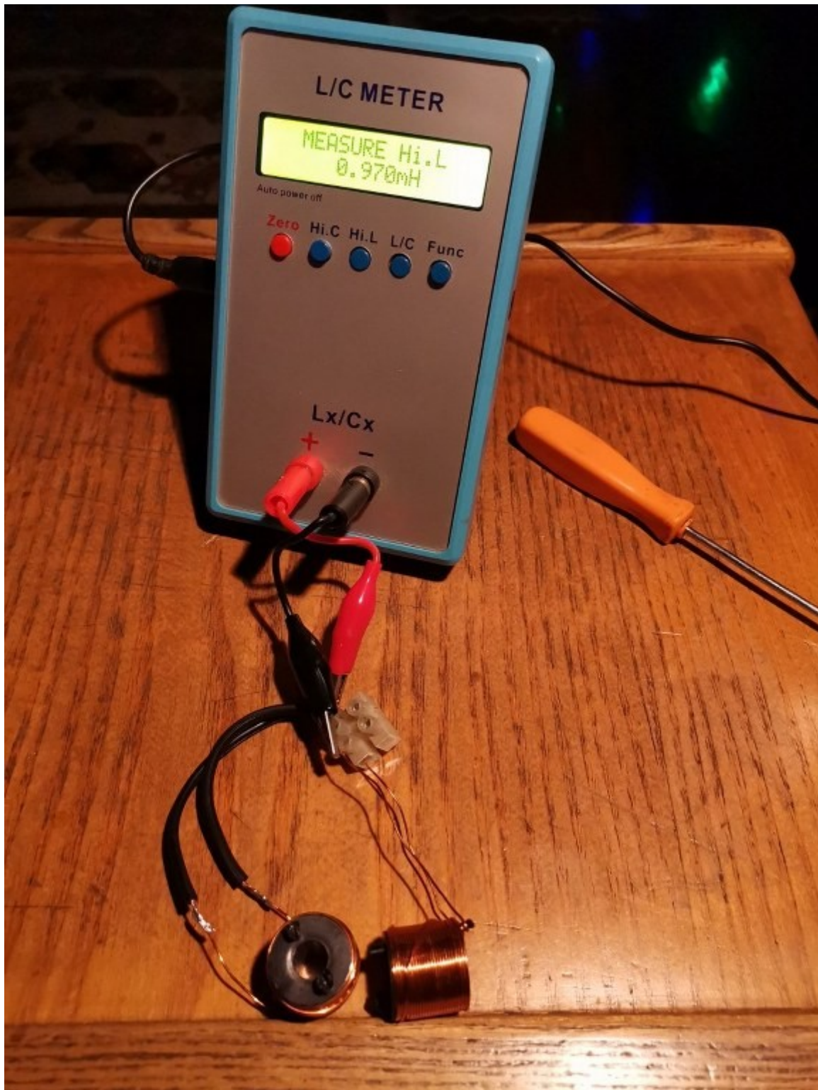
Figura 21: Coils close together, one reversed, perpendicular axis, 0,970mH.
