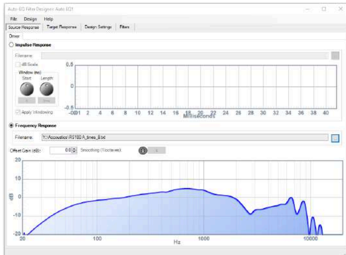
Figuur 53 Laden frequentie response in Sigmastudio in Automatic EQ block
