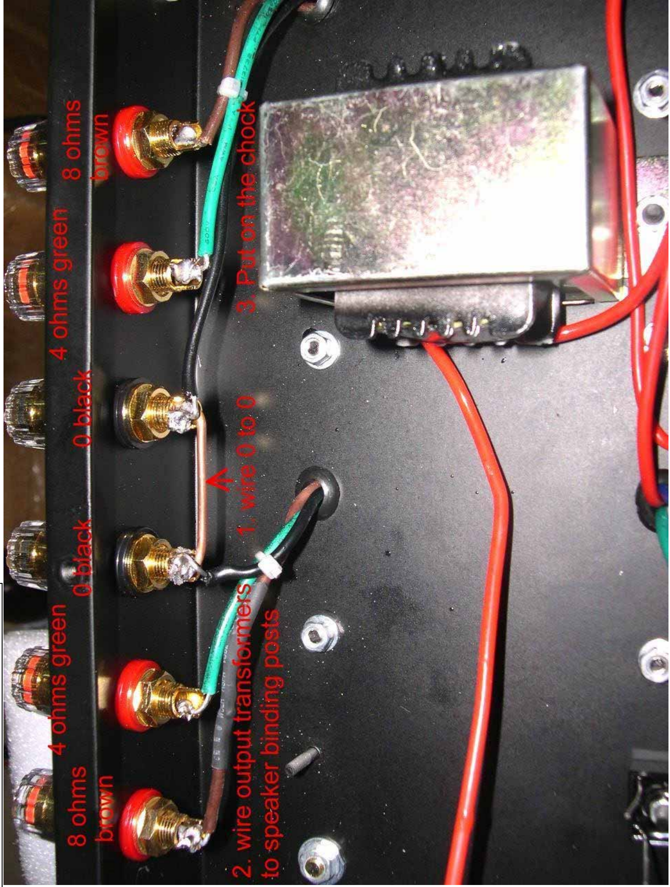
Step 6. Speaker binding posts wiring and choke loading;
